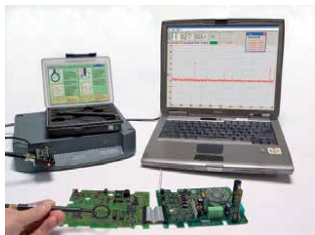
Measurements with the HX0083 proximity probe up to 10 cm from the target
