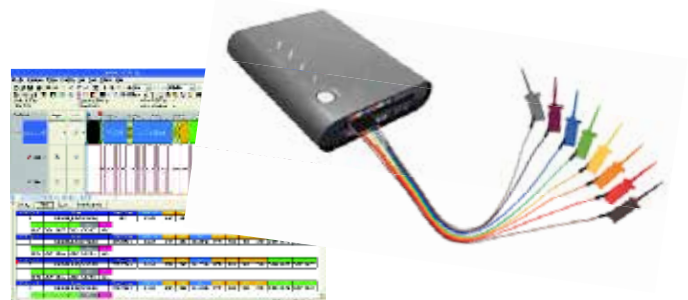
Self-contained bus-decoding probe powered via USB
